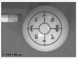
The first thing that catches the eye is the difference in the size of the contact spot at the moment of maximum compression of the tip. For Kamui Black H, the contact spot is about 5 - 6 mm in diameter, while for Rocket it is as big as 10 mm.
