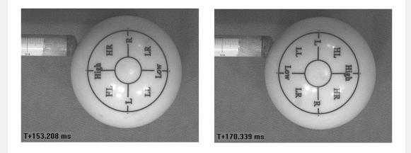
The second difference is the different duration of the contact of the cue and cue the ball. For Kamui Black H, the duration is 1.37 ms, for Rocket – 1.93 ms.
